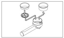
Place the pod inside the filter. Make sure that the edge of the pod does not extend over the rim of the filter basket.
