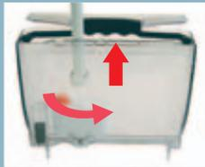
Turn the applicator counter-clockwise and remove it from the tank.
