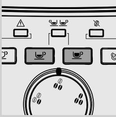
**4** The machine warms up and the “☕” and “☕” buttons blink. The “🔌” button turns off.
