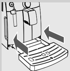
**4** Insert the drip tray with grill into the machine. Make sure it is fully inserted.
