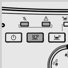
**13** The "💧" "⚠️" lights and the "☕" button light start to blink slowly to indicate that the water circuit needs to be primed.
