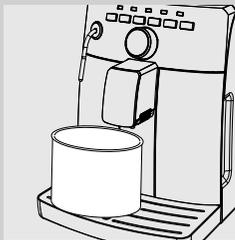
**6** Place a large container (1.5 l) under the steam/hot water wand and the dispensing spout.
