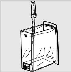
**4** Remove the water tank and pour the entire content of the Saeco descaling solution. Fill the water tank with fresh water up to the MAX level.
