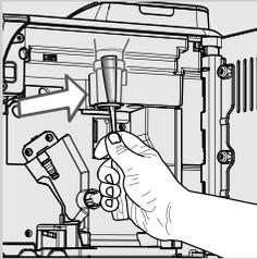
**5** Thoroughly clean the coffee outlet duct with the handle of a spoon or with another rounded kitchen utensil.
