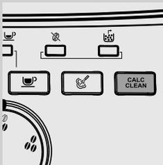
**7** Press and hold the "CALC CLEAN" button for 3 seconds. When the button starts blinking, release it to start the cycle. The "CALC CLEAN" button blinks during the whole descaling cycle.
