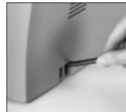
**3.4 Press the main ON/OFF switch.** After the automatic self-test, the **WARMING UP...** indicator will appear in the display.
