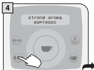
4 If desired, select the quantity of coffee to be ground by pressing the 000 button one or more times.
