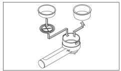
Place the pod inside the filter. Make sure that the edge of the pod does not extend over the rim of the filter basket.
