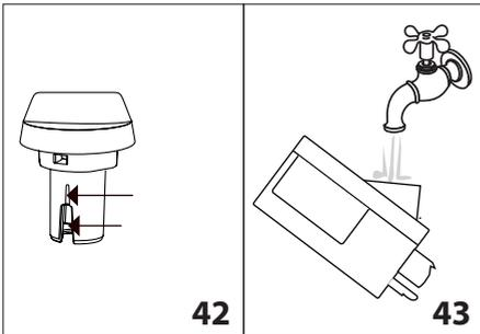
5. Rinse inside the froth adjustment dial seat with running water (fig. 43).
