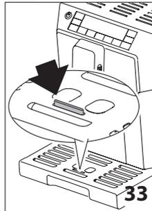
The drip tray (A12) is fitted with a level indicator (A13 - red) showing the level of water it contains (fig. 33). Before the indicator protrudes from the cup tray (A11), the drip tray must be emptied and cleaned, otherwise the water may overflow the edge and damage the appliance, the surface it rests on or the surrounding area.
