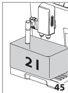
8. Place an empty container with a minimum capacity of 67,63 fl.oz/2.0 litres under the coffee spouts (A7) and hot water spout (C6) (fig. 45);
