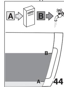
7. Pour the descaler into the tank up to level A (corresponding to a 3,38 fl.oz/ 100ml pack) marked on the inner surface of the tank (fig. 44), then add water (33,81 fl.oz/1 litre) up to level B (fig. 44) and put the water tank back.
