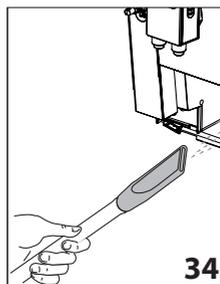
1. Check regularly (about once a week) that the inside of the appliance (accessible after removing the drip tray (A12) is not dirty. If necessary, remove coffee deposits with the brush (C5) supplied and a sponge.
