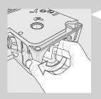
14 Turn the brew group back to the off position by manually turning the pin on the base, as shown in this figure. Turn it until it locks into the position described in the following step.
