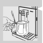
You need to perform a rinse cycle when using the machine for the first time. During this process, the coffee brewing cycle is activated and fresh water flows through the dispensing spout. This takes a few minutes.
