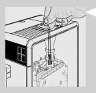
3 Thoroughly clean the pre-ground coffee compartment with the cleaning brush, making sure that there are no more coffee residues in the duct.
