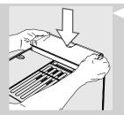
4 Insert the coffee bean hopper into its compartment as shown in the figure.
