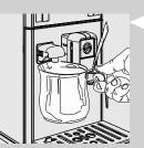
6 Dispense the desired amount of hot water. To stop the hot water dispensing, press the Special Beverages " button again.
