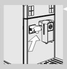
14 Check that the water dispensing spout is correctly installed.
