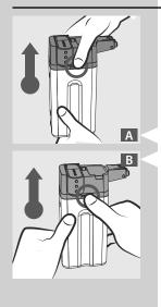
1 Press one of the release buttons to remove the top of the carafe as shown in the figures (A or B).
