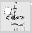
10 Pour one milk cleaner bag into the milk carafe. Fill the milk carafe with fresh drinking water up to the MAX level and then let the milk cleaner bag dissolve completely.
