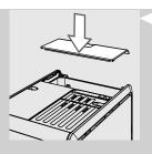
3 After removing it, put the protection lid on the machine.
