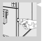
1 Press the button in the frame and open the service door.
