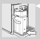
3 Push the carafe towards the bottom while rotating it at the same time, until it is locked onto the drip tray.
