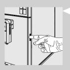
4 Press the button in the frame and open the service door.
