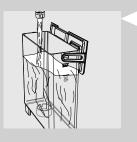
7 Fill the water tank with fresh water up to the CALC CLEAN level.
