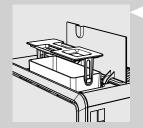
6 Remove the water tank by using the handle incorporated on the inner
