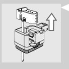
3 Lift the carafe dispenser to remove it from the top of the carafe. The carafe dispenser is made up of six parts that must be disassembled. Each part is indicated by a capital letter (A, B, C, D, E, F).
