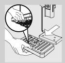
7 Press the lever on the bottom and remove the drip tray (external), empty it and wash it.
