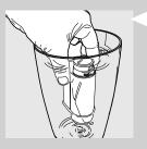
1 Remove the "INTENZA+" water filter from its packaging, immerse it vertically (with the opening positioned upwards) in cold water and gently press the sides so as to let the air bubbles out.
