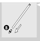
5 Remove the fitting (B) from the suction tube.
