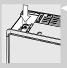
2 Clean the coffee compartment with a cloth to remove any coffee residues and dust.
