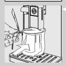
9 Place a container (1.5 l) under the coffee dispensing spout. Press the "\sqrt{"}" button to start the cleaning cycle.
