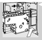
16 Insert the brew group back into its seat by sliding it along the guides until it locks into place.
